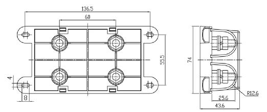
Insulating Body : Nylon With Glass Fiber / PC Applicable : For ANL 25A~200A
