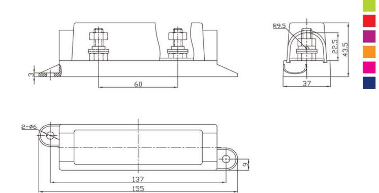
Insulating Body : Nylon With Glass Fiber / PC Applicable : For ANL 25A~200A
